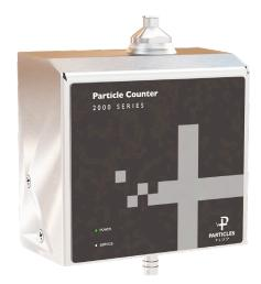
The 2301 and 2501 particle counters provide a range of particle size measurement from 0.3 or 0.5 to 25.0  $\mu$ m at a flow rate of 0.1 CFM (2.83 LPM). These sensors allow for efficient particle counting with specifications that exceed the ISO 21501-4 and JIS B9921 calibration standards.
