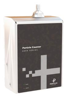
The 2301P and 2501P particle counters provide a range of particle size measurement from 0.3 to 25.0  $\mu$ m at 0.1 CFM (2.83 LPM) flow. These sensors allow for efficient particle counting with high accuracy and resolution that meet or exceed ISO 21501-4 and JIS B9921 for the calibration of a particle counter.
