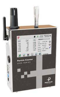
The Particles Plus<sup>®</sup> 5300P Remote Particle Counter measures 0.3  $\mu$ m to 25.0  $\mu$ m with a flow rate of 1.2 LPM and is the most versatile remote particle counter available.
