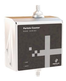
The 9301 and 9501 Modbus particle counters provide a range of particle size measurement from 0.3 to 25.0  $\mu$ m at a flow rate of 0.1 CFM (2.83 LPM). These sensors allow for efficient particle counting with specifications that exceed the ISO 21501-4 and JIS B9921 calibration standards.
