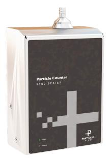
The 9510 Modbus particle counters provide a range of particle size measurement from 0.5 to 25.0  $\mu$ m at a flow rate of 1.0 CFM (28.3 LPM). These sensors allow for efficient particle counting with specifications that exceed the ISO 21501-4 and JIS B9921 calibration standards.
