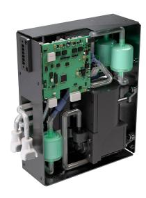
The 15000-OEM condensation particle counter (CPC) is designed to detect and count aerosol particles by first enlarging the particulates using a supersaturated vapor. These robust monitors provide reliable, accurate measurement of airborne nanoparticles across a very wide size range allowing for the detection of environmental and public health concerns involving airborne particulates.
