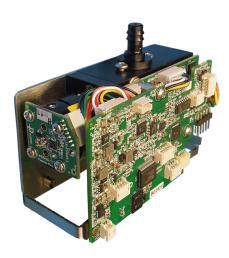
The 2300-OEM particle sensor provides a range of particle size measurement from 0.3 to 25.0  $\mu$ m at 1.2 LPM flow. These sensors allow for efficient particle counting with high accuracy and resolution that meet or exceed ISO 21501-4 and JIS B9921 for the calibration of a particle counter.
