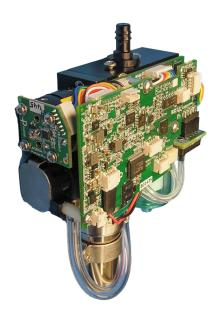
The 2300P-OEM particle counter provides a range of particle size measurement from 0.3 to 25.0  $\mu$ m at 1.2 LPM flow. These sensors allow for efficient particle counting with high accuracy and resolution that meet or exceed ISO 21501-4 and JIS B9921 for the calibration of a particle counter.
