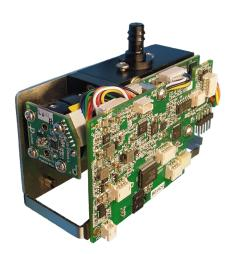
The 2301-OEM particle sensor provides a range of particle size measurement from 0.3 to  $25.0~\mu m$  at 0.1 CFM (2.83 LPM) flow. These sensors allow for efficient particle counting with high accuracy and resolution that meet or exceed ISO 21501-4 and JIS B9921 for the calibration of a particle counter.
