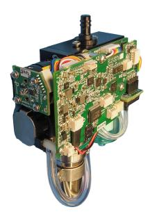
The 2301P-OEM particle counter provides a range of particle size measurement from 0.3 to 25.0  $\mu$ m at 0.1 CFM (2.83 LPM) flow. These sensors allow for efficient particle counting with high accuracy and resolution that meet or exceed ISO 21501-4 and JIS B9921 for the calibration of a particle counter.
