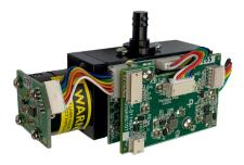
The Particles Plus<sup>®</sup> 4300-OEM is a laser-based particle sensor that uses the light scattering method to detect and count particles in any given indoor or outdoor environment. The 4300-OEM measures particles from 0.3 to 25.0  $\mu$ m. The sensor is ideal to detect the concentration of particles precisely in real-time. The unit includes a particle sensor, particle counter board and operates from 9-15 VDC.
