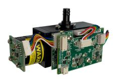
The Particles Plus® 4301-OEM is a laser-based particle sensor that uses the light scattering method to detect and count particles in any given indoor or outdoor environment. The 4301-OEM measures particles from 0.3 to 25.0  $\mu$ m. The sensor is ideal to detect the concentration of particles precisely in real-time. The unit includes a particle sensor, particle counter board and operates from 9-15 VDC.
