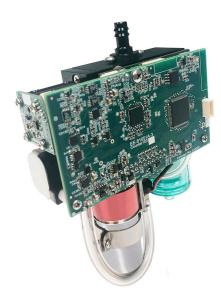
The 9300P-OEM measures up to 30 channels of particle count data from 0.3 to 25.0 µm with a flow rate of 1.2 LPM. The assembly is mounted on a plate for ease of integration. The unit includes a particle sensor, particle counter board, integrated vacuum pump and manifold with pre/post filters, real-time clock/calendar with battery backup, logging and data storage for up to 65,000 sample records, communicates via UART and operates from 7-15 VCD.
