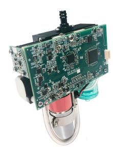
The 9301P-OEM measures up to 30 channels of particle count data from 0.3 to 25.0 µm with a flow rate of 2.83 LPM. The assembly is mounted on a plate for ease of integration. The unit includes a particle sensor, particle counter board, integrated vacuum pump and manifold with pre/post filters, real-time clock/calendar with battery backup, logging and data storage for up to 65,000 sample records, communicates via UART and operates from 7-15 VCD.
