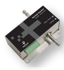
The Particles Plus® 2510-4 Remote Particle Counter measures 0.5  $\mu$ m, 0.7  $\mu$ m, 1.0  $\mu$ m & 5.0  $\mu$ m with a flow rate of 1.0 CFM (28.3 LPM). Integration is easy into a realtime monitoring or building management system via Modbus MRTU. The 2510 is the smallest 1.0 CFM remote particle counter on the market and has easy mounting options. The Particles Plus® 2510-4 complies with ISO 21501-4 and includes a 1 year limited warranty.
