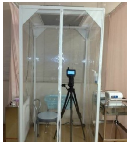
Fig.1 Nebulizer and OPC setting in clean booth.
