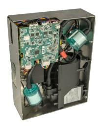
The 15000-OEM condensation particle counter (CPC) is designed to detect and count aerosol particles by first enlarging the particulates using a supersaturated vapor. These robust monitors provide reliable, accurate measurement of airborne nanoparticles across a very wide size range allowing for the detection of environmental and public health concerns involving airborne particulates.
