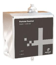
The 2301 and 2501 particle counters provide a range of particle size measurement from 0.3 or 0.5 to 25.0  $\mu$ m at a flow rate of 0.1 CFM (2.83 LPM). These sensors allow for efficient particle counting with specifications that exceed the ISO 21501-4 and JIS B9921 calibration standards.
