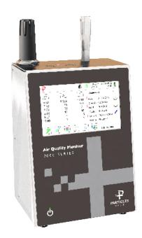
The Particles Plus® 7300 Remote Particle Counter measures  $0.3 \mu m$  to  $25.0 \mu m$  with a flow rate of 1.2 LPM and is the most versatile remote particle counter available.
