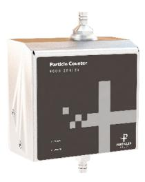
The 9510 particle counters provide a range of particle size measurement from 0.5 to 25.0  $\mu$ m at a flow rate of 1.0 CFM (28.3 LPM). These sensors allow for efficient particle counting with specifications that exceed the ISO 21501-4 and JIS B9921 calibration standards.
