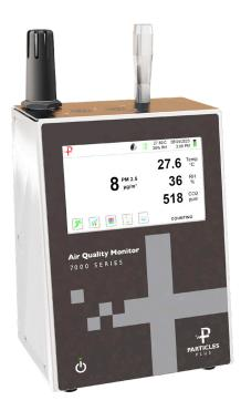
The Particles Plus 7300-AQM1 and 7300-AQM2 Remote Particle Counters measure particles from 0.3 to 25.0  $\mu$ m at a flow rate of 1.2 LPM. These user-friendly instruments display up to six particle size channels, temperature, relative humidity, and CO<sub>2</sub> (AQM1) or CO<sub>2</sub> + TVOC (AQM2).
