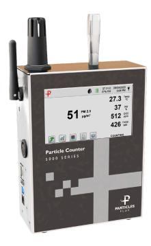
The Particles Plus® 5300-AQM1 and 5300-AQM2 Remote Particle Counters measure particles from 0.3 to 25.0  $\mu$ m. These user-friendly instruments display up to six particle size channels, temperature, relative humidity, and CO $_2$  (AQM1) or CO $_2$  + TVOC (AQM2). Featuring a 1.2 LPM flow rate, the 5300 is optimized for high-concentration environments providing improved accuracy, reduced coincidence loss, and extended instrument lifespan in comparison to higher-flow models.
