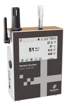
The Particles Plus® 5301-AQM1 and 5301-AQM2 Remote Particle Counters measure particles from 0.3 to 25.0  $\mu$ m at a flow rate of 0.1 CFM (2.83 LPM). These user-friendly instruments display up to six particle size channels, temperature, relative humidity, and CO<sub>2</sub> (AQM1) or CO<sub>2</sub> + TVOC (AQM2).
