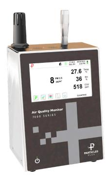
The Particles Plus® 7300-AQM1 and 7300-AQM2 Air Quality Monitors measure particles from 0.3 to 25.0 µm. These user-friendly instruments display up to six particle size channels, temperature, relative humidity, and CO<sub>2</sub> (AQM1) or CO<sub>2</sub> + TVOC (AQM2). Featuring a 1.2 LPM flow rate, the 7300 is optimized for high-concentration environments providing improved accuracy, reduced coincidence loss, and extended instrument lifespan in comparison to higher-flow models.
