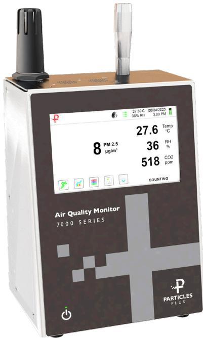
The Particles Plus® 7300-AQM1 and 7300-AQM2 Remote Particle Counters measure particles from 0.3 to 25.0 µm at a flow rate of 1.2 LPM. These user-friendly instruments display up to six particle size channels, temperature, relative humidity, and CO<sub>2</sub> (AQM1) or CO<sub>2</sub> + TVOC (AQM2).
