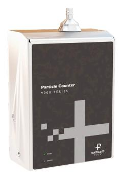
The Particles Plus® 9300P Remote Particle Counters are designed for continuous monitoring in cleanrooms and other controlled environments. With 30 user-selectable particle size channels ranging from 0.3 up to 25.0 µm and a quiet 1.2 LPM internal pump, these instruments deliver targeted contamination detection with real-time data collection and configurable alarms for immediate incident reporting and local visual alerts.
