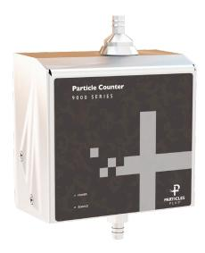
The Particles Plus® 9301 and 9501 Remote Particle Counters are designed for continuous monitoring in cleanrooms and other controlled environments. With 30 user-selectable particle size channels ranging from 0.3 or 0.5 up to 25.0 µm and a flow rate of 0.1 CFM (2.83 LPM), these instruments deliver targeted contamination detection with real-time data collection and configurable alarms for immediate incident reporting and local visual alerts.
