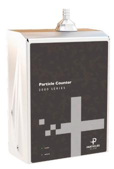
The Particles Plus® 2301P and 2501P Remote Airborne Particle Counters are designed for continuous monitoring in cleanrooms and other controlled environments. With four particle size channels ranging from 0.3 or 0.5 up to 25.0 µm, these instruments deliver targeted contamination detection with real-time data collection and configurable alarms for immediate incident reporting and local visual alerts.
