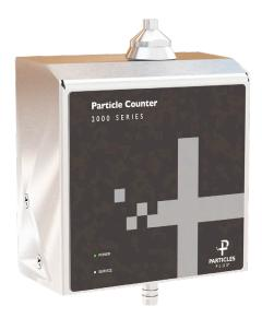
The Particles Plus® 2510 and 2510-2 Remote Particle Counters provide a range of particle size measurement from 0.5 to 25.0  $\mu$ m at a flow rate of 1.0 CFM (28.3 LPM) and are designed for continuous monitoring in cleanrooms and other controlled environments. With two or four particle size channels, these instruments deliver targeted contamination detection with real-time data collection and configurable alarms for immediate incident reporting and local visual alerts.
