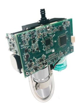
The Particles Plus® 9300P-OEM Airborne Particle Counters feature a minimalist design to maximize functionality for researchers and OEM applications with 30 user-selectable particle size channels ranging from 0.3 up to 25.0 µm. Featuring a 1.2 LPM flow rate, the 9300P-OEM is optimized for high-concentration environments providing improved accuracy, reduced coincidence loss, and extended instrument lifespan in comparison to higher-flow models.
