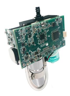
The Particles Plus® 9301P-OEM Airborne Particle Counters feature a minimalist design to maximize functionality for researchers and OEM application, with 30 user-selectable particle size channels ranging from 0.3 up to 25.0  $\mu$ m at a 0.1 CFM (2.83 LPM) flow rate.
