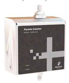
Particles Plus® 9510 Remote Airborne Particle Counters monitor particle sizes ranging from 0.5 to 25  $\mu$ m across six user-selectable channels at a flow rate of 1.0 CFM (28.3 LPM). These instruments are designed for collecting particle data in cleanrooms or other controlled environments, and seamlessly integrate with Particles Plus® Software, facility monitoring systems, or local data collection platforms.
